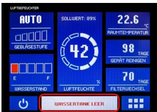
Fig. 7.2.1: Fault display on the touch display
