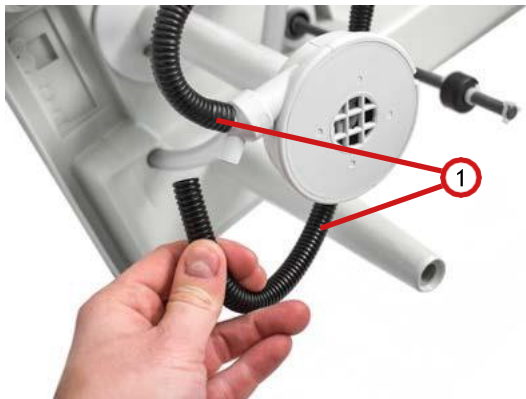
Fig. 6.3.4.4: Pulling off the pump hoses
