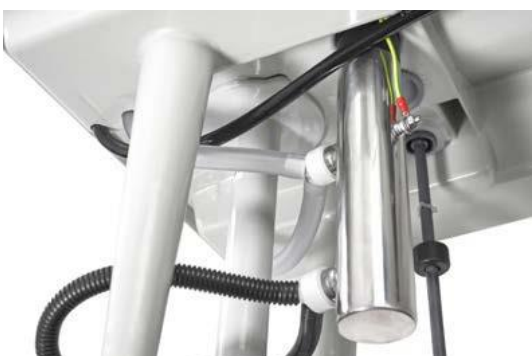
Fig. 8.1.2.8: UV disinfection unit, complete
