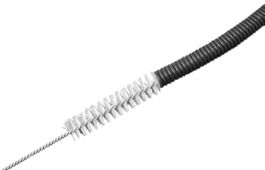
Fig. 6.3.4.5: Cleaning the pump hoses
