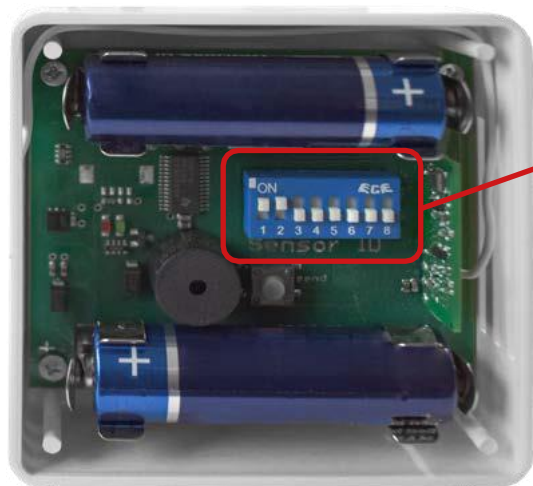
Fig. 5.6.1: Interior view of radio humidity transmitter
