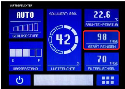
Fig. 5.1.6: Next recommended cleaning display
