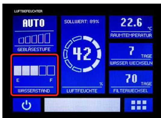
Fig. 5.1.2: Water level display
