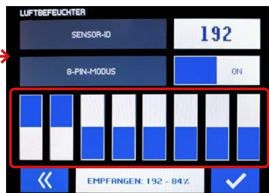
Fig. 5.6.7: Coding radio humidity transmitter
