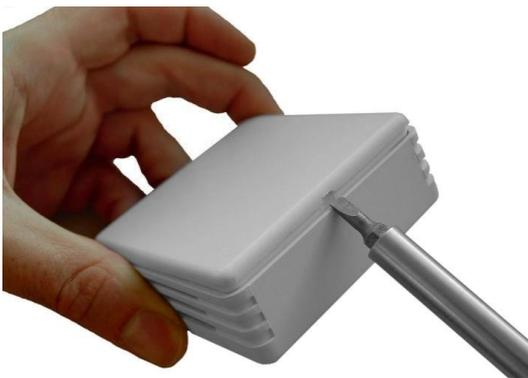
1. Carefully lift the cover of the radio humidity transmitter with a small screwdriver and remove it (fig. 3.4.1).
