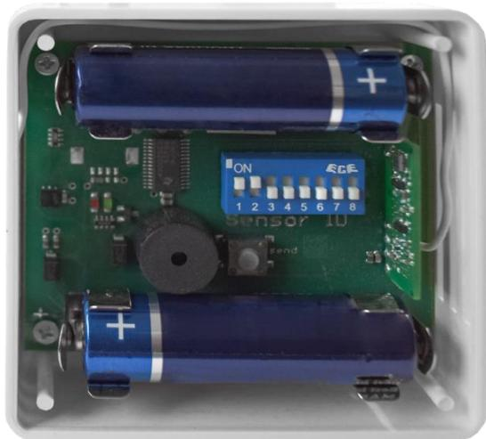
Fig. 3.5.1: Coding switch for coding
