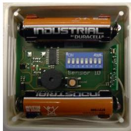
Fig. 17: Coding the wireless sensor system
