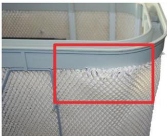
*Fig. 10: Incorrect filter placement*
