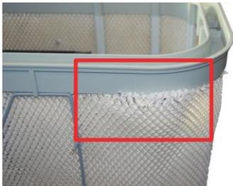
Fig. 30: Incorrect filter placement
