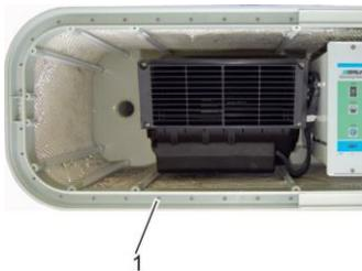
Fig. 24: Cleaning the drainage holes
