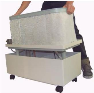
Fig. 34: Removing the center piece
