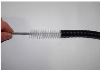
Fig. 39: Cleaning the pump hoses
