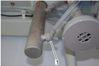
Fig. 68: Cleaning the stainless steel pipe
