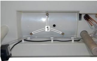
Fig. 54: Removing bolts
