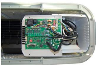
Fig. 73: Removing the control panel
