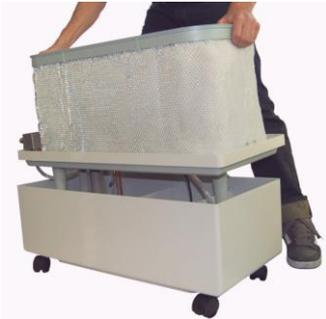
Fig. 65: Removing the center piece
