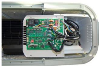
*Fig. 20: Removing the control panel*
