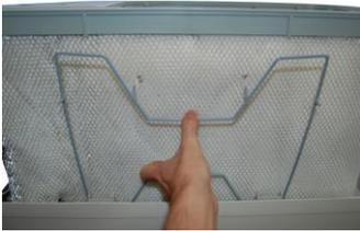
Fig. 28: Removing the filter bracket
